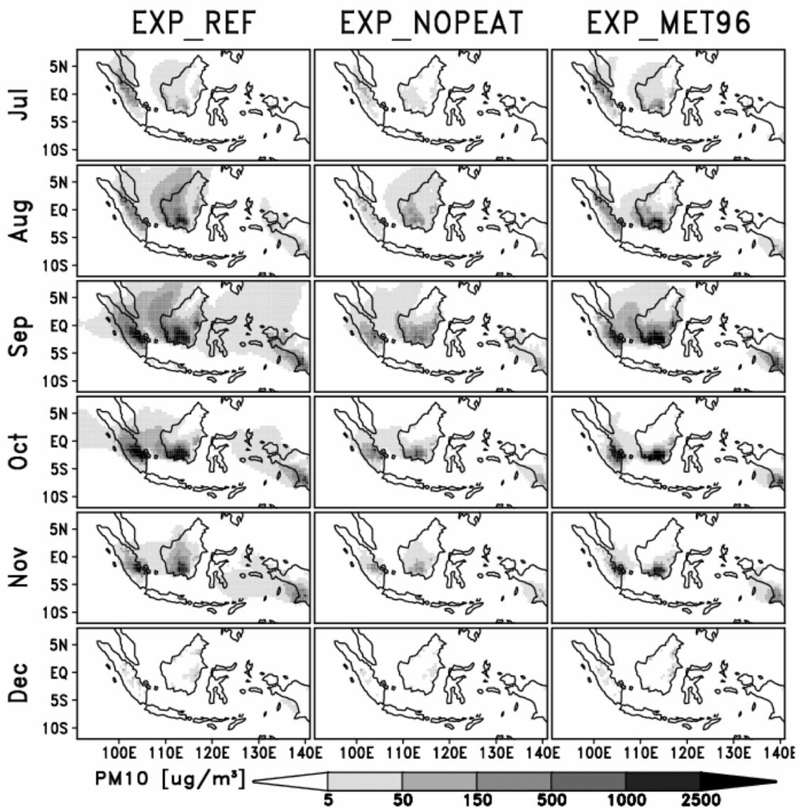
Figure 2. Monthly mean  $PM_{10}$  concentration during 1997 modelled with REMOTE for the lowest model layer for the scenario runs EXP\_REF (left column), EXP\_NOPEAT (middle column) and EXP\_MET96 (right column).
