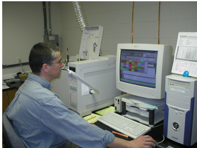
Figure 2. Real-life photo of Aroma Trax™ MDGC-olfactometry system.
