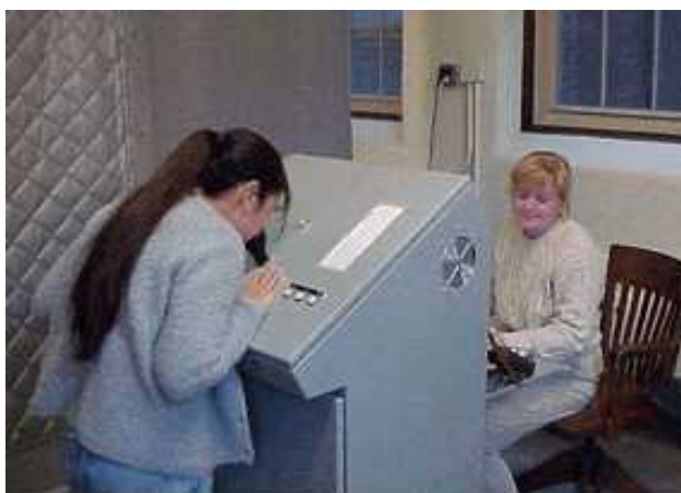
Figure 3. AC'SCENT® International Olfactometer in use by sniffer and panel leader.
