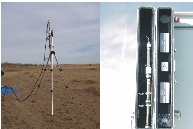
Figure 1. Typical URG sampler setup at upwind (left photo) and downwind (right photo) dairy locations.
